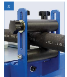
CENTERING DEVICE GUIDA TUBO
